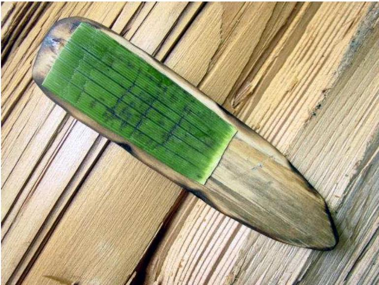
Here's a nifty sanding invention that utilizes a strip of horsetail (*Equisetum hyemale*), which I glued to a piece of Yellow Cedar with deer hide glue. This works well at finish sanding.
